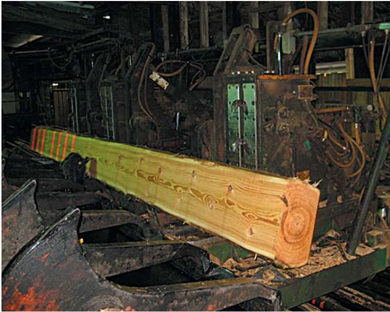
A Western Red Cedar log is milled on the headrig at Mary's River Lumber.
